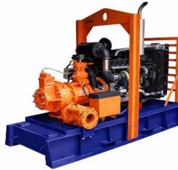
Godwin HL125M Diesel Driven, Automatic Self-priming Pump Flow up to 300m 3 /h and head to 134m
