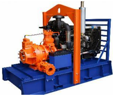
Godwin HL125M Diesel Driven, Automatic Self-priming Pump Flow up to 300m 3 /h and head to 134m
